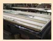
Salem floor joists support a 5/8" Tongue and Groove, residential grade plywood floor system....
